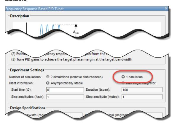
The Frequency Response Based PID Tuner is particularly useful when PID Tuner cannot linearize the plant at the operating point you want to use for tuning. For more information, see Frequency-Response Based Tuning.
